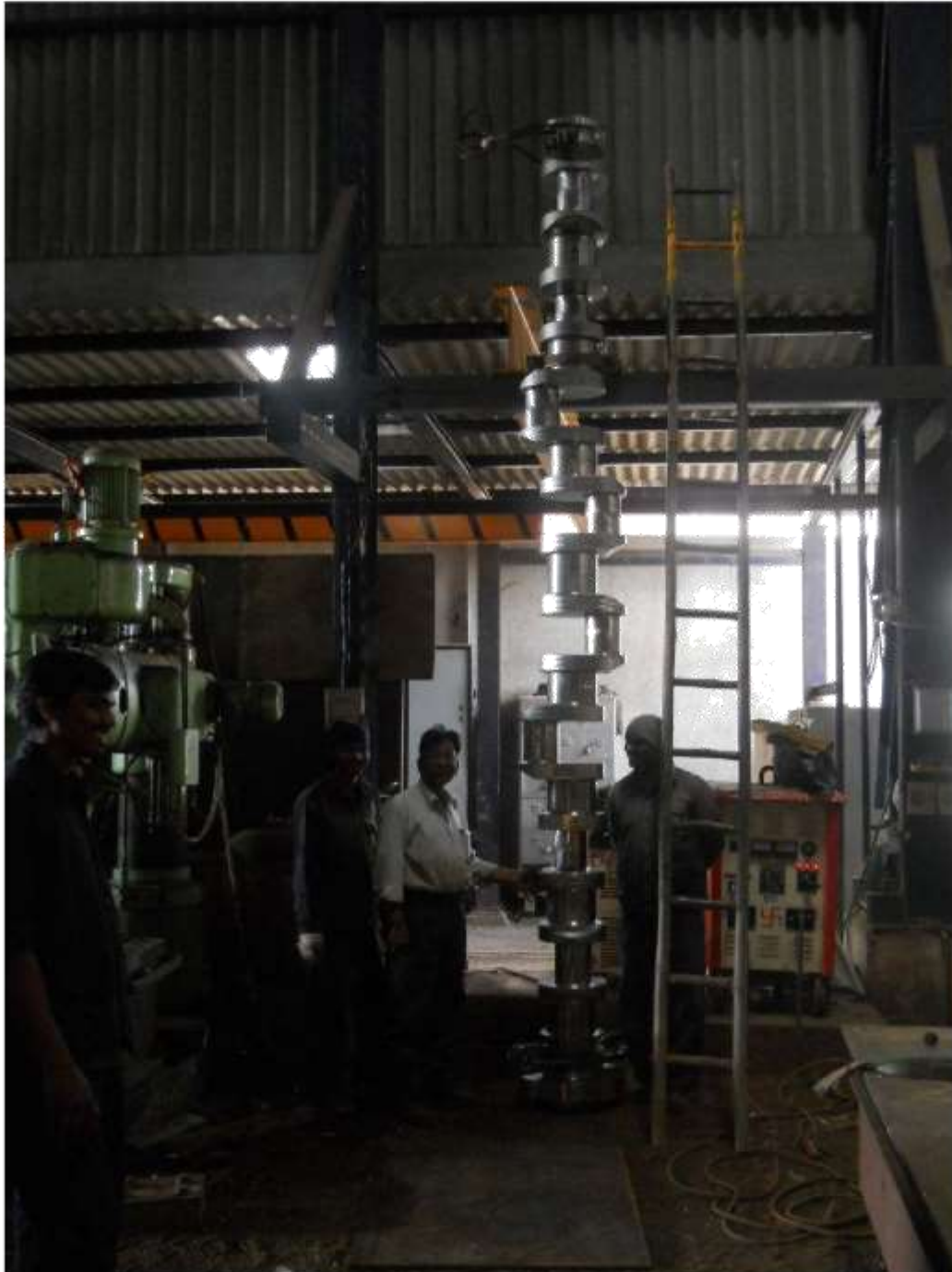
COUNTERWEIGHT WELDING ON LOCOMOTIVE CRANKSHAFT
