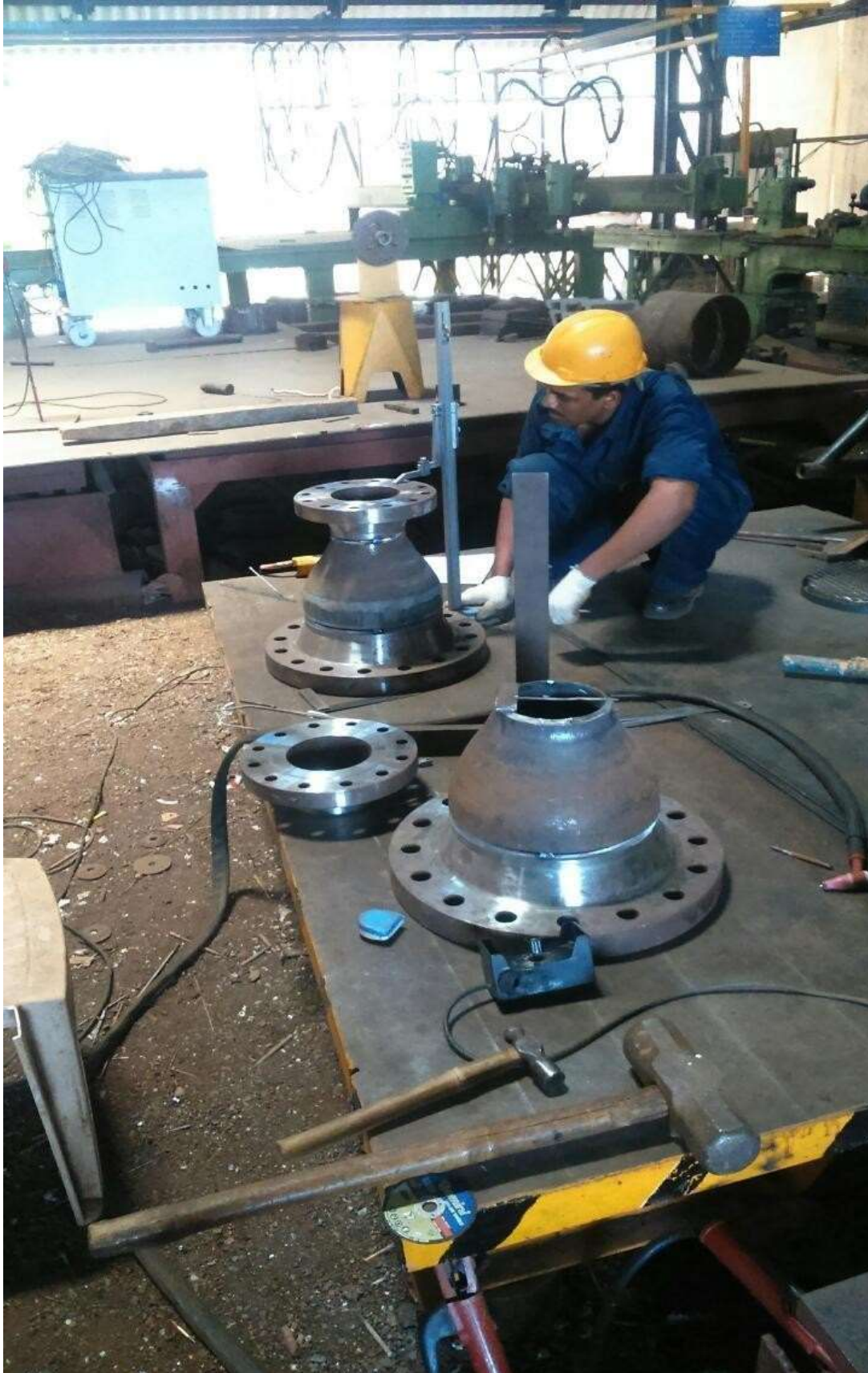
FABRICATION & SUPPLY OF SPOOL PIECES TO KSB PUMPS LTD (IBR & NON IBR) MATERIALS A105 & SS316L
