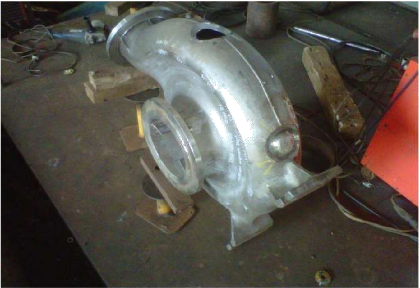
WINDOW WELDING ON A GLOBAL PUMP
