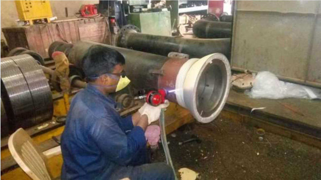
Aluminium Bronze Thermal Spraying on Suspension Body
