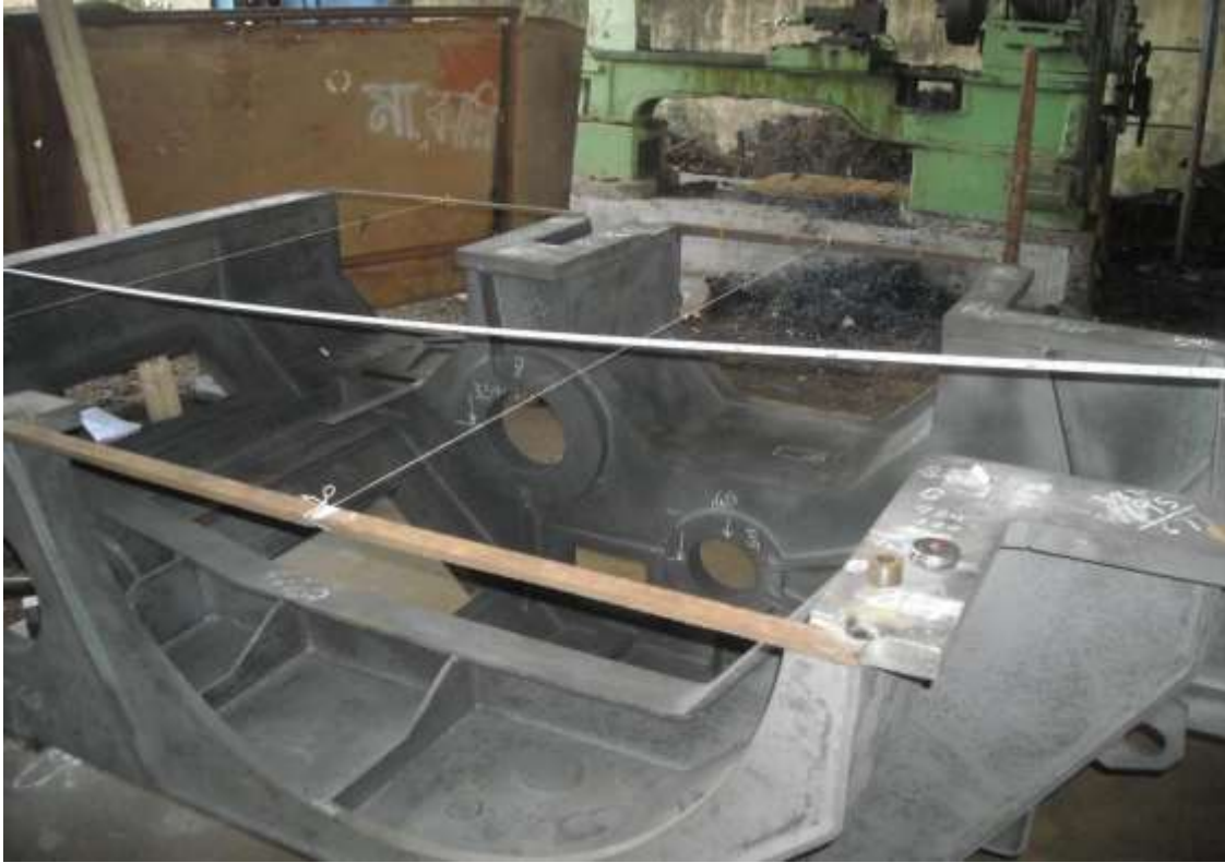
Fabrication of NOPV Gear boxes under Inspection of ABS & IRS
