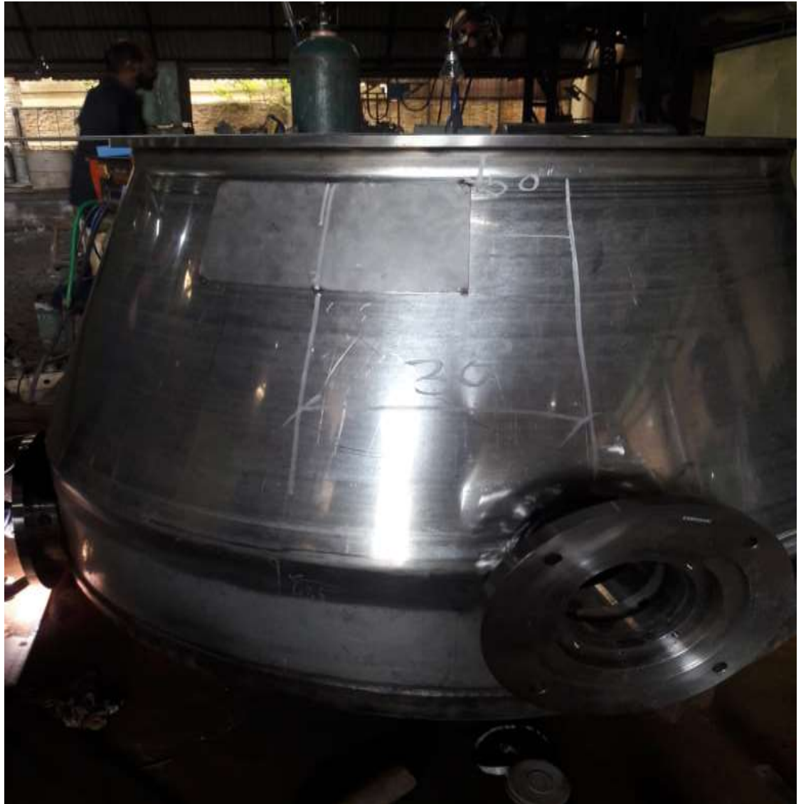
Stainless Steel Fabrication and Welding for Pharma Equipments (Product Bowl)
