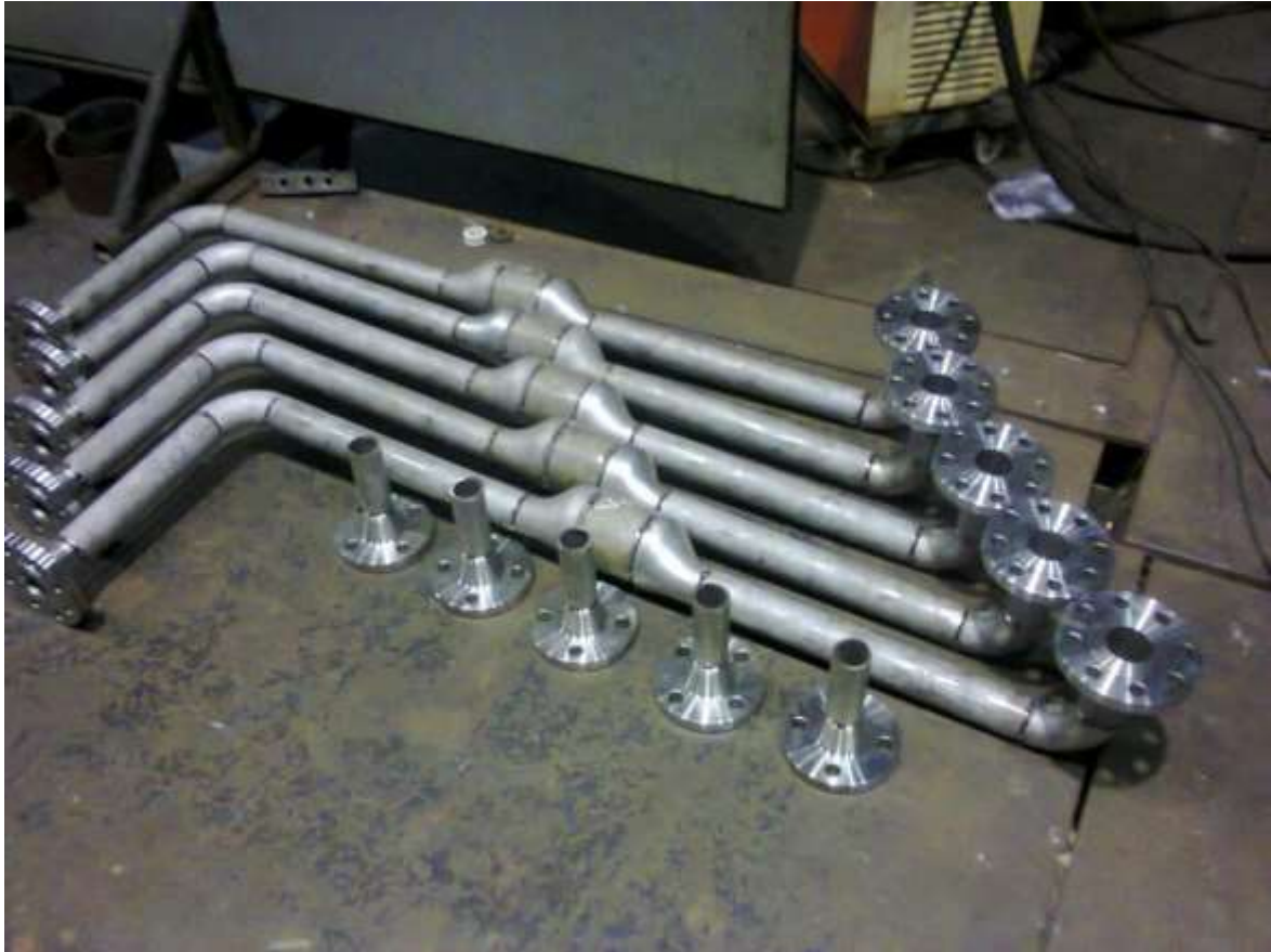
FABRICATION OF BALANCING LINE PIPING FOR KSB PUMPS AS PER IBR1950
