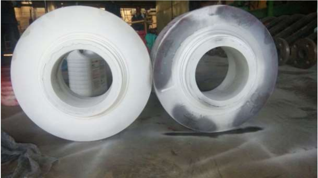
SS316L & Inconel 625 Overlay on Ball Valve Bodies
