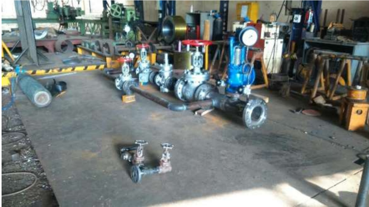
FABRICATION & ASSEMBLY OF PRESSURE REDUCING STATION (PRS)
