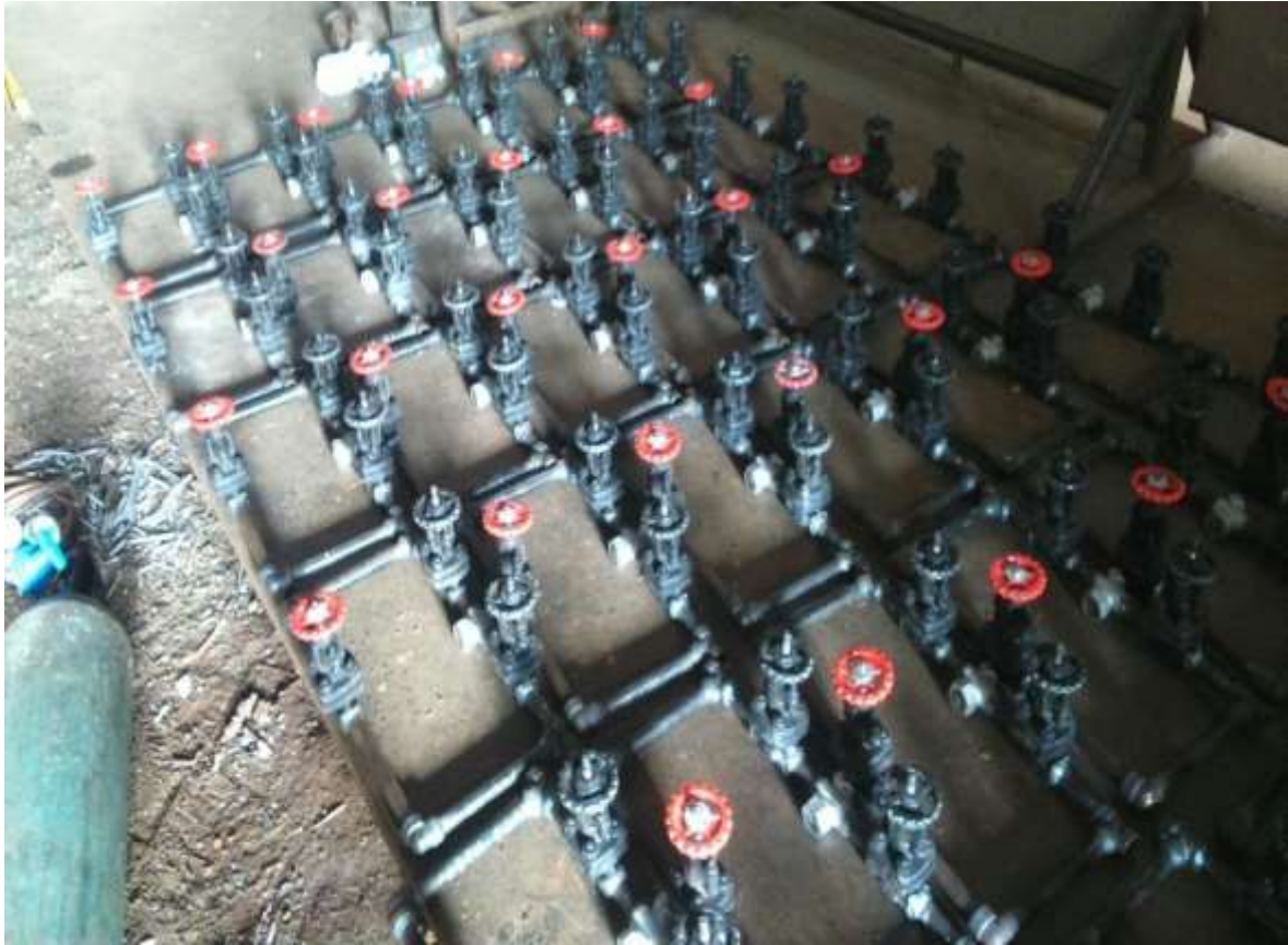
FABRICATION & SUPPLY OF STEAM TRAP MODULES AS PER IBR 1950
