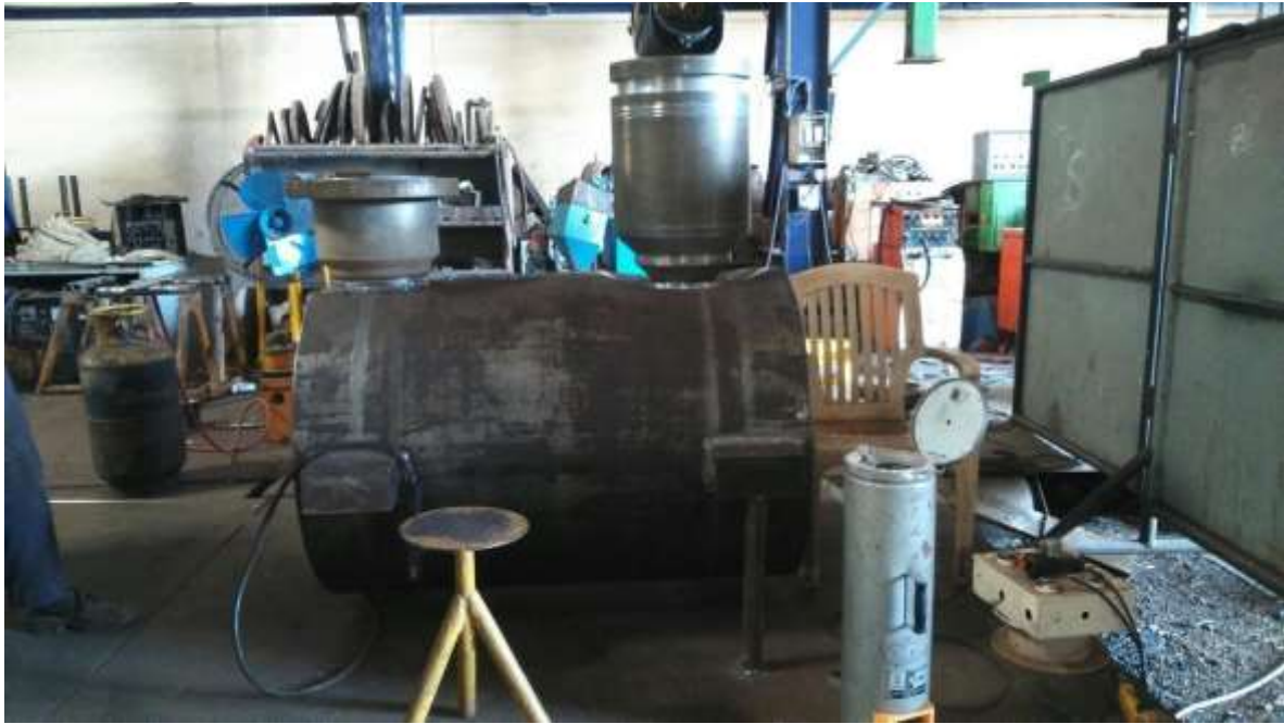
NOZZLE WELDING ON PUMP BARREL CASING
