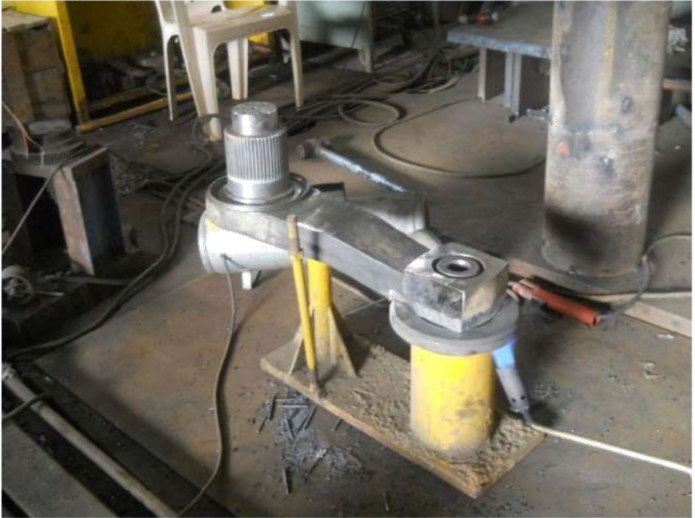
AXLE ARM WELDING OF ARJUN TANKS
