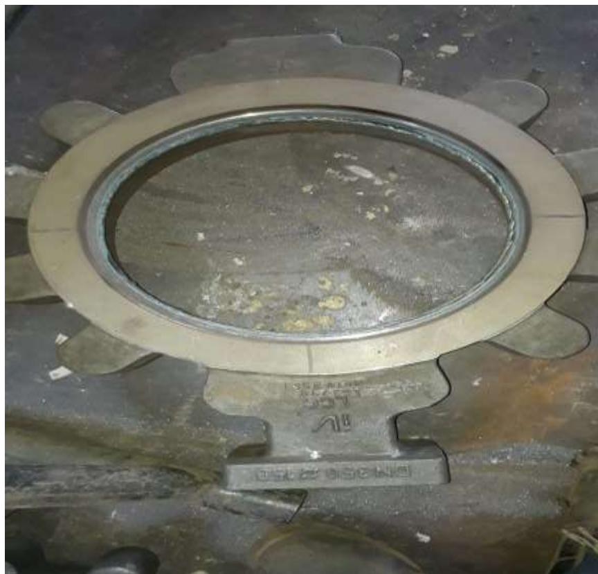
Stellite 21 overlay on Butterfly Valve bodies
