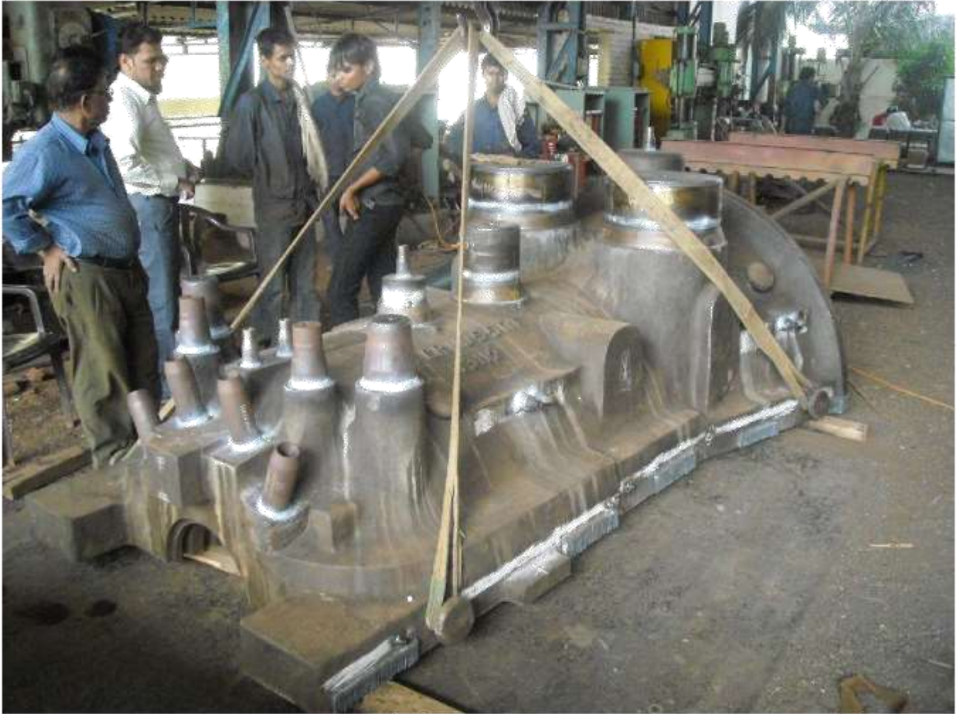
NOZZLE WELDING ON A TURBINE CASING
