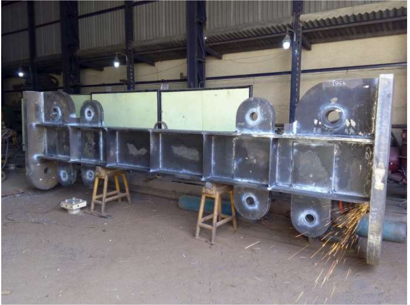
Fabrication of Lifting Beam of Lifting Capacity 250 MT(Self Weight 7MT)
